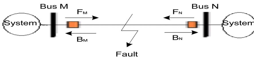
Fig. 1. Diagram for single phase transmission line
