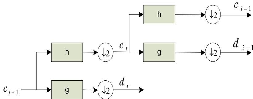
Fig. 2. Diagram of MRA decomposition into two scales
