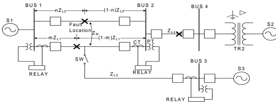
Fig.4. One-line diagram of IEEE EMTP reference model
