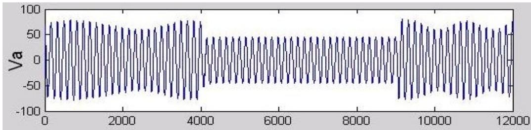
Fig.5. Typical voltage waveform for a symmetrical fault during power swing
