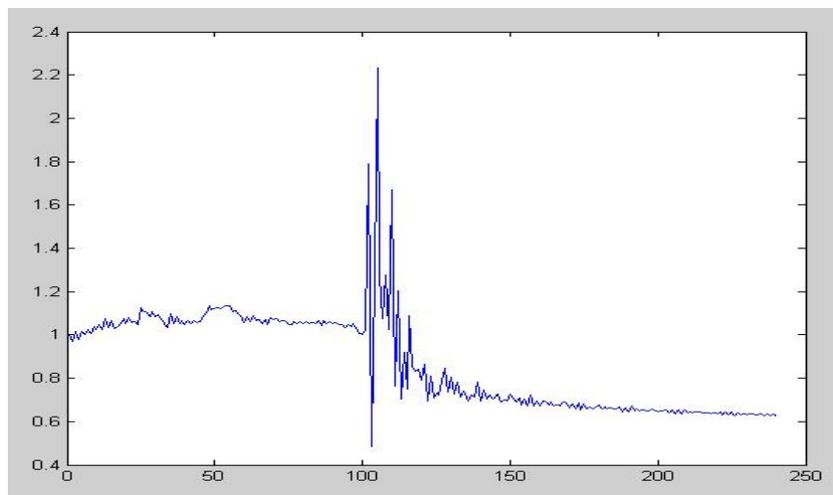
Fig.6. Values of criteria factor  $k_e$  around the fault point
