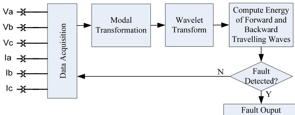
Fig. 3. Implementation diagram of symmetrical fault detection during power swing
