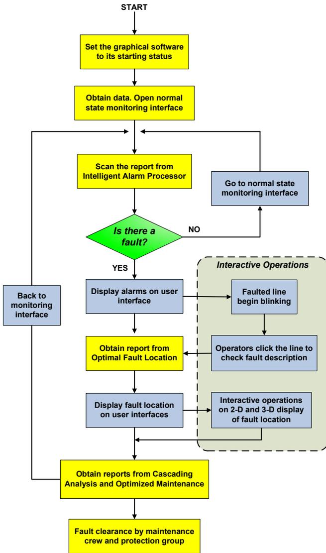
Fig. 7: Implementation Flow Chart of the Software
