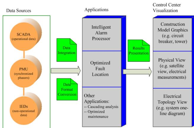
Fig. 2: Data sources, applications and control center visualization options
