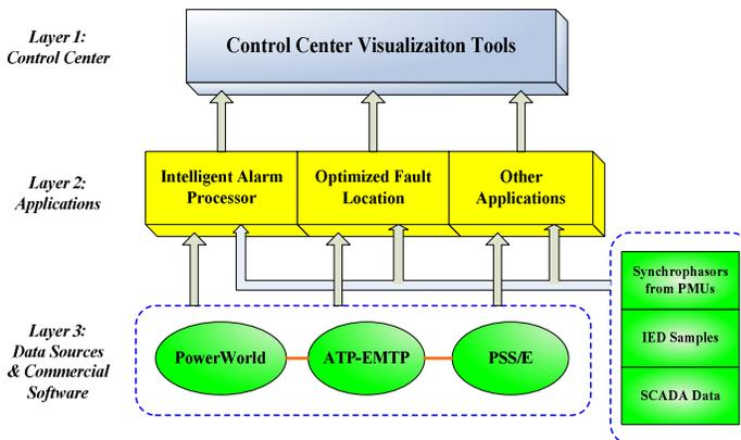
Fig. 3: Hierarchy of the visualization system
