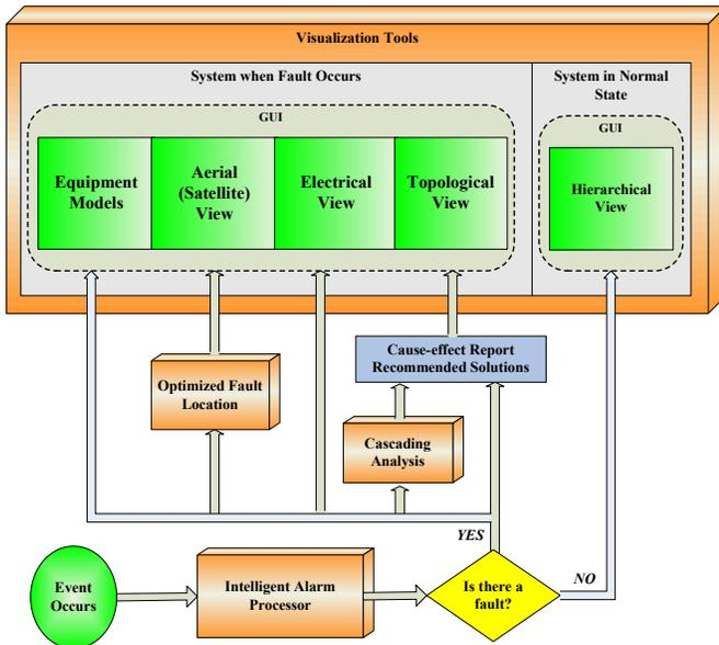
Fig. 4: Functions of Visualization Tools
