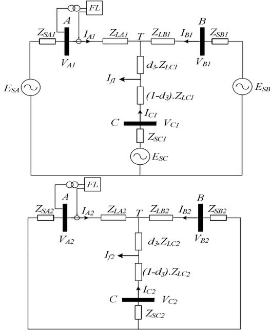
Figure 3. Positive and negative sequence diagram for fault in section T-C.
