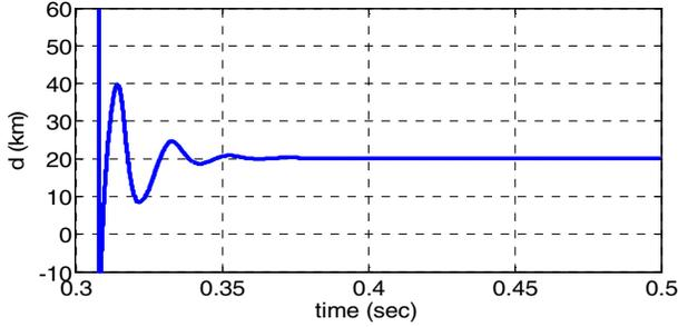
Figure 5. ab-g fault with 50Ω resistance 20km from bus A at section A-T.
