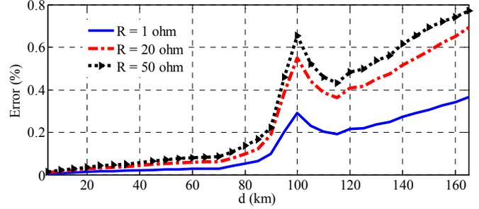
Figure 7. Fault location error versus distance, during an abc-g fault along sections A-T and T-C for three different fault resistances.
