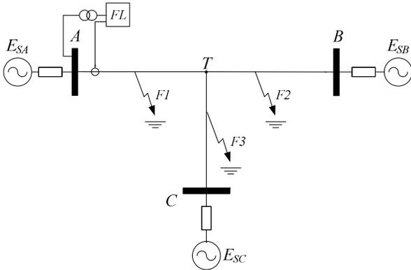
Figure 1. A typical three-terminal transmission line.
