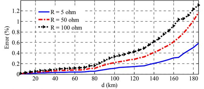
Figure 8. Fault location error versus tapped point distance from Bus A during an ac-g fault at the middle point of section T-C for three different fault resistances.
