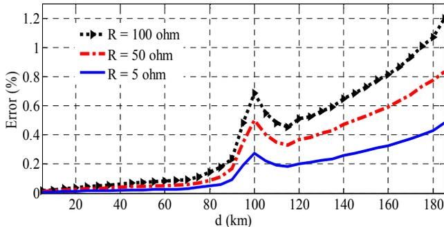
Figure 6. Fault location error versus distance, during a c-g fault along sections A-T and T-B for three different fault resistances.
