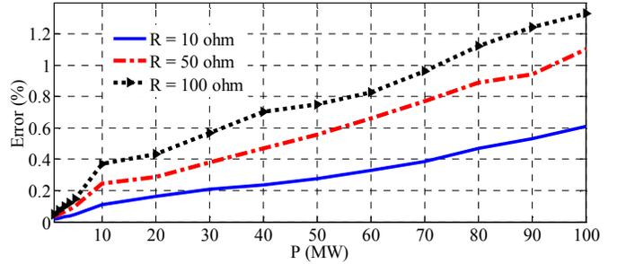
Figure 9. Fault location error versus tapped end (bus C) active power during an a-g fault at the middle point of section T-B for three different fault resistances.
