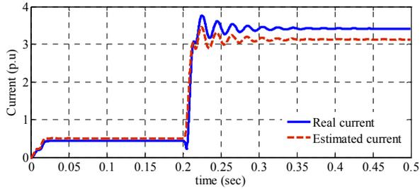
Figure 10. Effect of source impedance variation on current estimation.
