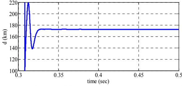
Figure 4. a-g fault with 20Ω resistance 170km from bus A at section B-T.
