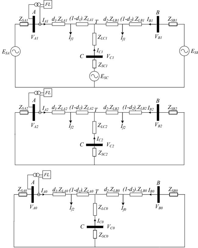
Figure 2. Positive, negative and zero sequence diagram for fault in section A-T or T-B.
