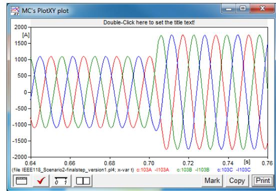
Fig. 9. Scenario-2: current waveforms from the ATP simulation
