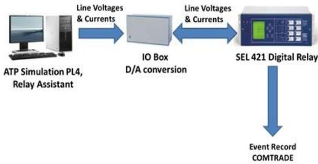
Fig. 6. Schematic of cascade scenario experimental test bench
