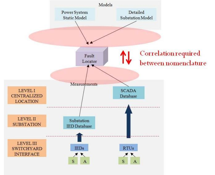
Fig. 4. Data and information flow for fault location application
