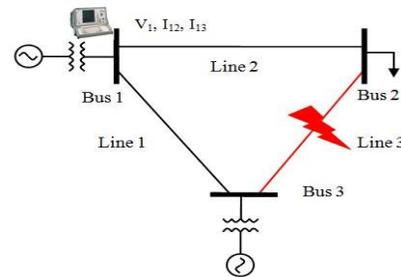
Fig. 7. One-line diagram of 3 bus power network
