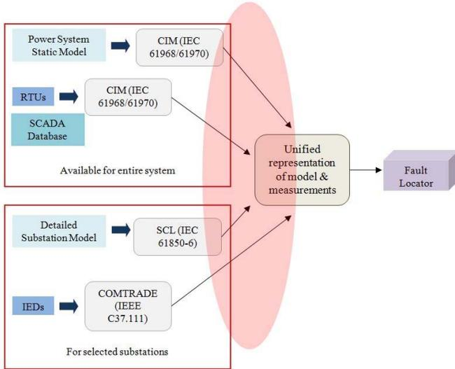
Fig. 5. Unified representation of data and model for fault location application
