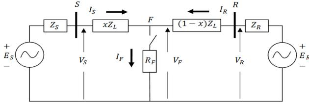
Fig. 2. Faulted circuit model
