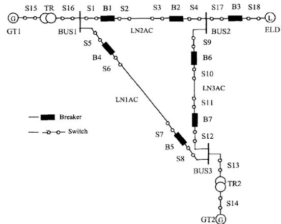
Fig. 6. Node breaker representation of 3 bus power network [22]
