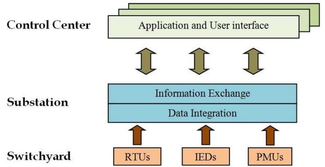
Fig. 1. Data flow in a substation
