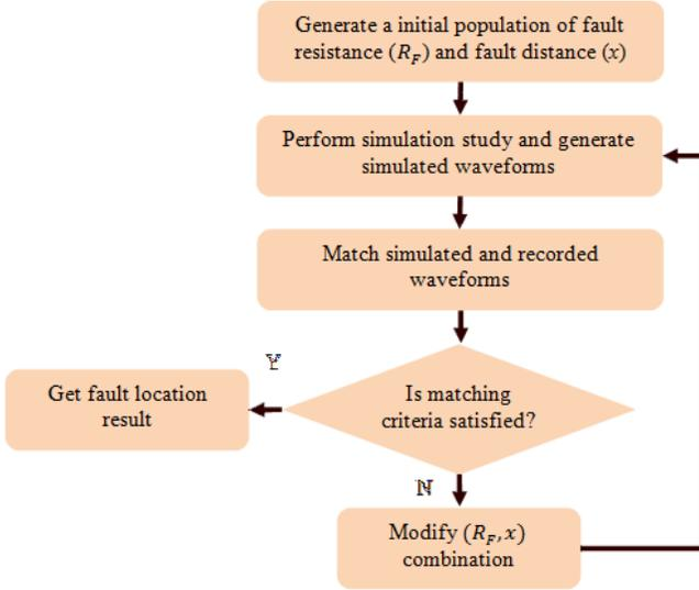
Fig. 3. Flowchart of sparse measurement algorithm
