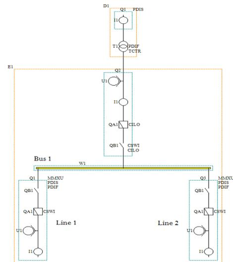
Fig. 8. Node breaker representation of Substation-1
