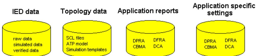
Figure 2 Database structure of the ASA
