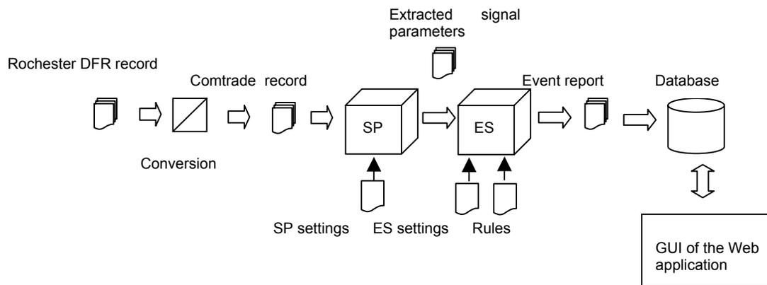
**Figure 6 CBMA software architecture**
