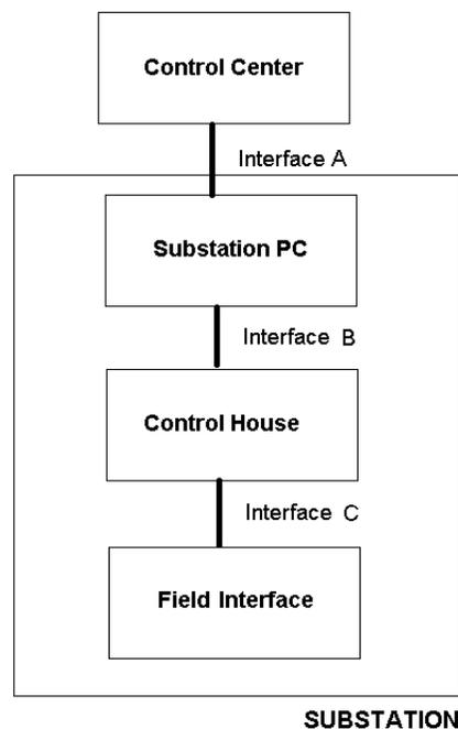
**Figure 3 IED Layers and interfaces of communication infrastructure in the substation**
