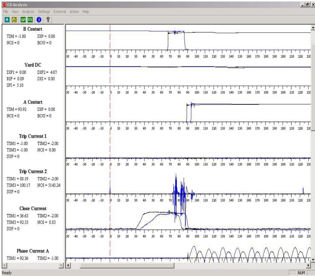
Figure 10 CBM signal waveforms displayed using CBMA Viewing software
