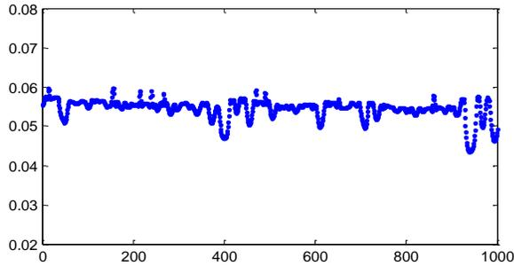
Figure 10. Damping ratios estimated from ambient measurements
