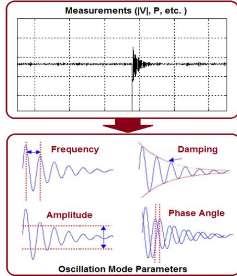
Figure 1. Mode parameters identified from power system measurements
