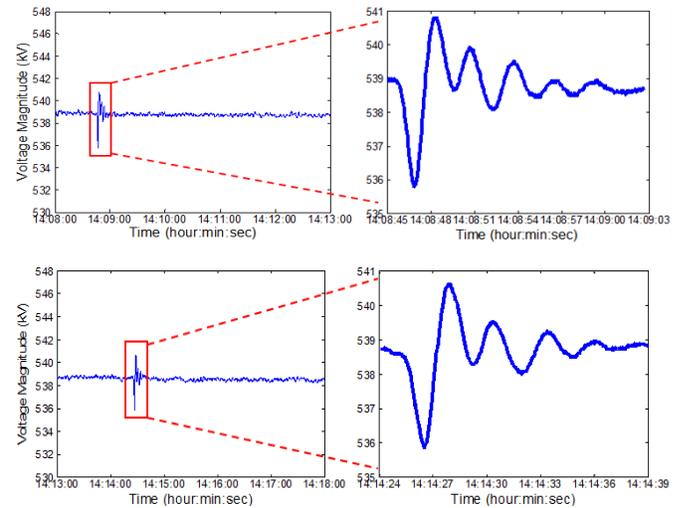
Figure 11. Field voltage magnitude measurements from PMUs
