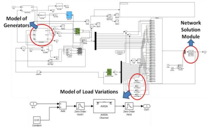
Figure 7. Simulink model of the IEEE 39-bus test system
