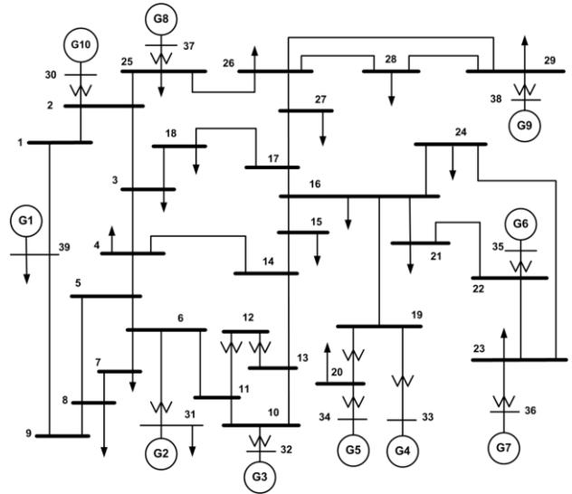
Figure 6. One-line diagram of IEEE 39-bus test system
