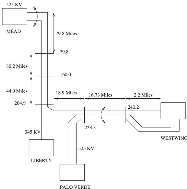
Fig. 3. One Line Diagram of the Sample Power System
