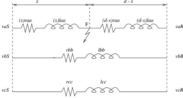
Fig. 1. Short Three Phase Tr. Line with Ph. A to Ground Fault
