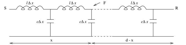
Fig. 2. Unfaulted Long Transmission Line
