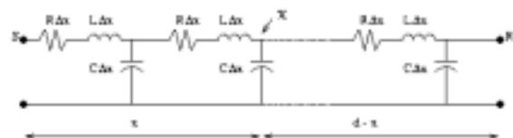
Figure 2: Unfaulted Long Transmission Line
