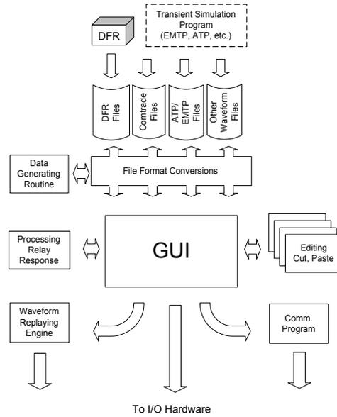
Fig. 10. The software architecture of the simulator
