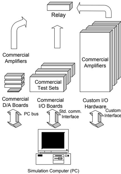
Fig. 9. The hardware architecture of the simulator
