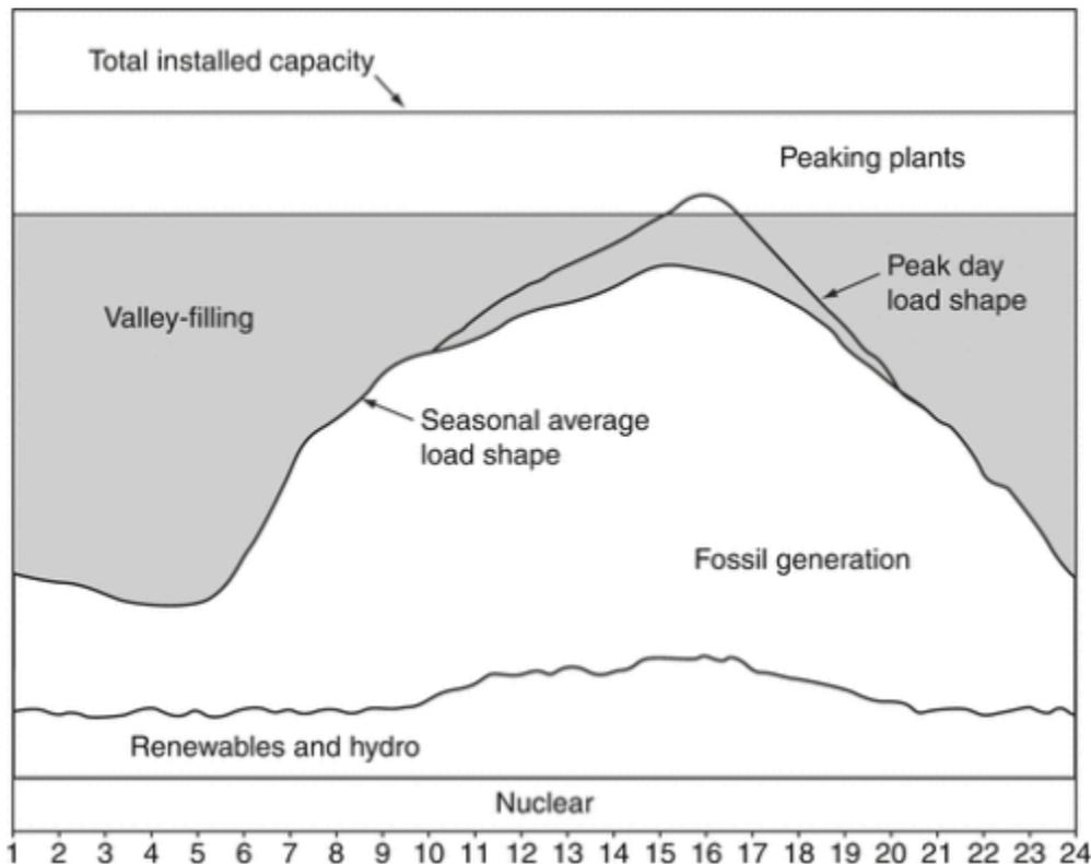
PHEVs and BEVs in Coupled Power and Transportation Systems. Figure 4 Illustrative peaking of electricity load [12]
