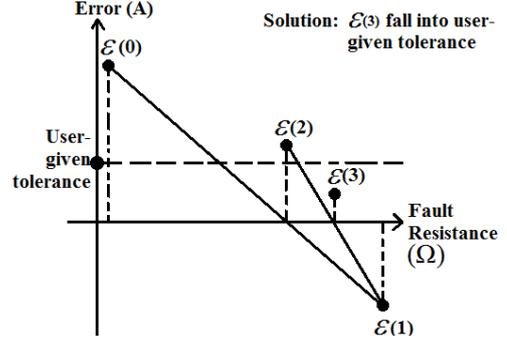
Figure 3. Fault resistance estimation procedure [19].
